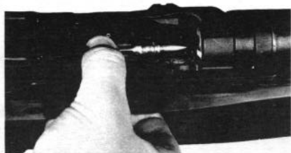
Figure 27. Loading the magazine with a single round (magazine in rifle).
