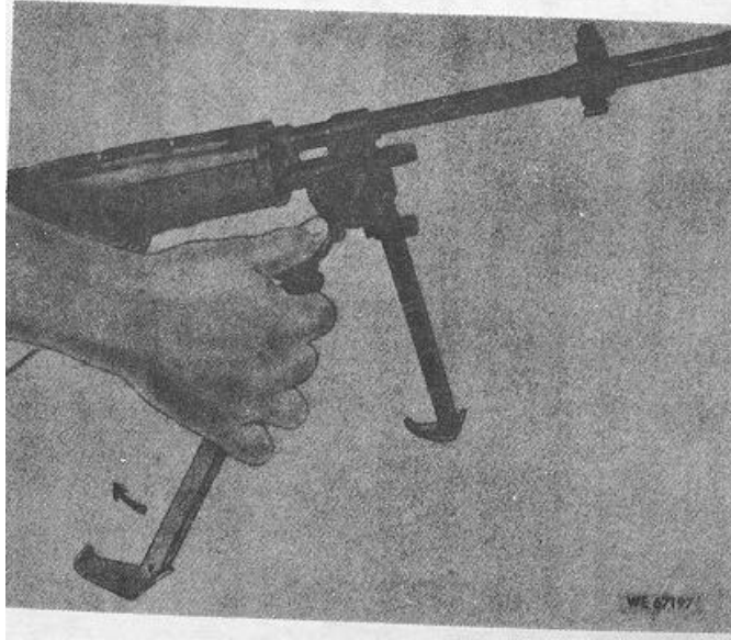
Figure 2-14. Adjusting bipod legs.
